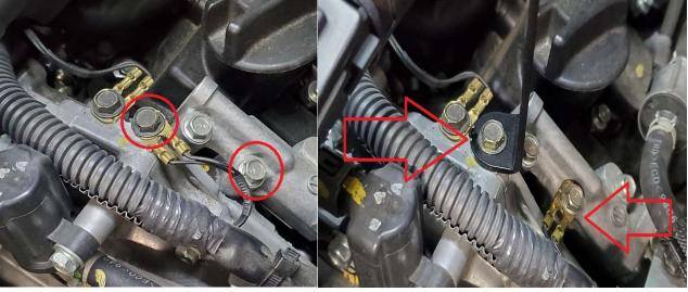
4 Locate PCV line on passenger side of engine, running from the intake manifold to the back of the engine. Squeeze clamps to slide them back and remove line.
